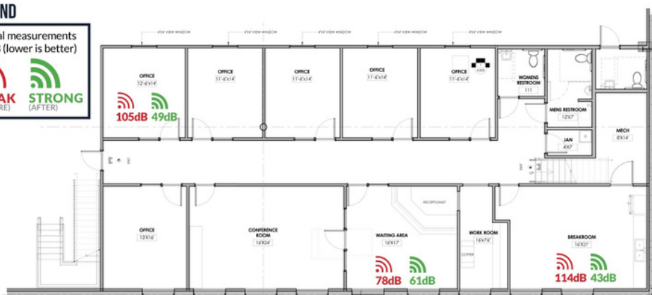
BEFORE AND AFTER LTE/5G CELLULAR SIGNAL AUDIT
