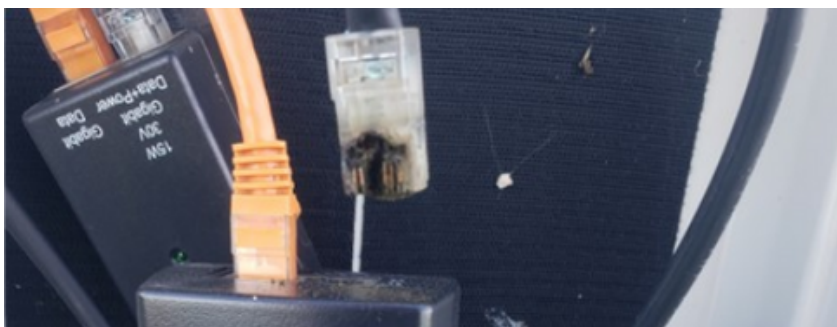
Fried ethernet connectors from old WiFi network
