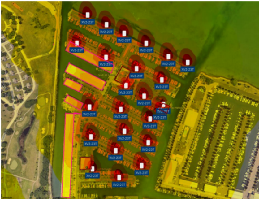
Metro Wireless's WiFi coverage heatmap design for MacRay Harbor
